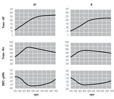
A1 = High performance crafts. Full throttle operation restricted within 10% of total use period. Cruising speed at engine rpm < 90% of rated speed setting - Maximum useage 300 hours per year.
