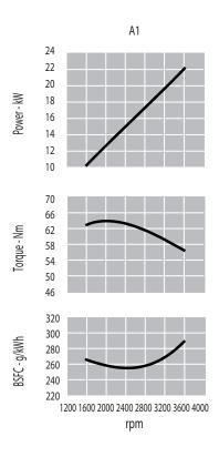
A1 = High performance crafts: Full throttle operation restricted within 10% of total use period. Cruising speed at engine rpm <90% of rated speed setting - Maximum useage 300 hours per year.
