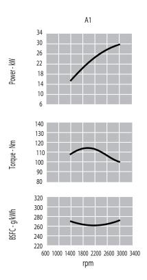
A1 = High performance crafts: Full throttle operation restricted within 10% of total use period. Cruising speed at engine rpm <90% of rated speed setting - Maximum useage 300 hours per year.
