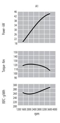
A1 = High performance crafts: Full throttle operation restricted within 10% of total use period. Cruising speed at engine rpm <90% of rated speed setting - Maximum useage 300 hours per year.
